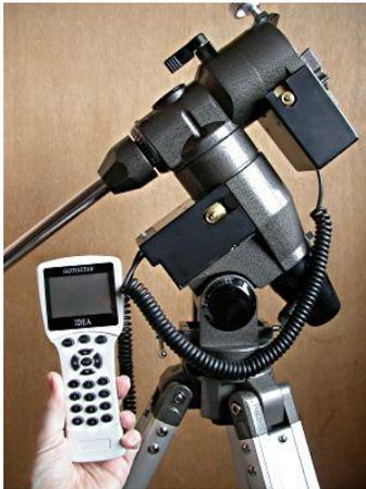
The telescope fits into the dovetail slot and the handset enables the object required to be entered, either by name or by RA and Dec. Press the OK button and off goes the telescope and finds the object you want. Wonderful! The descriptions and manuals are all on the [loptron](#) and [Astronomica](#) websites.
