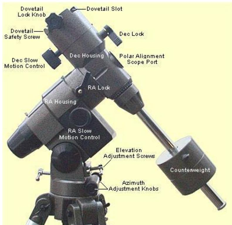
By fitting motors to each drive (RA and Dec) and having a GoTo handset and computer, all the sweat can be taken out of directing the telescope to where you want to be. The expert star-hoppers in the Society will be horrified at this suggestion, but this is the system I'm describing and, until I can learn to star-hop with a good telescope, it gets me along!
